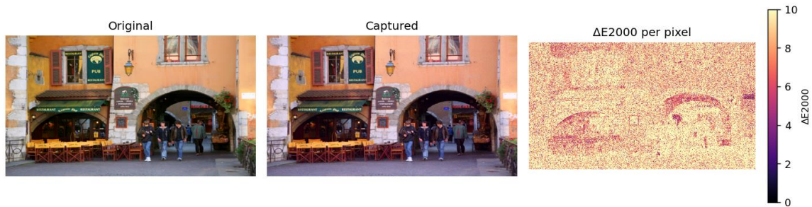
Figure 15.2 — Original frame, captured frame (with hue shift), and per-pixel \Delta E2000 heatmap.
