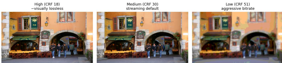
Figure 13.1 — Same source frame at the three quality presets. CRF 18 is visually transparent, CRF 30 is the streaming default, CRF 51 introduces visible artefacts.
