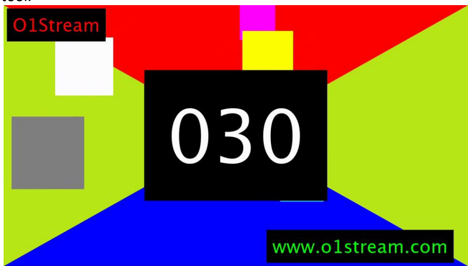
Figure 13.11 — One frame from frame_counter_60Hz.mp4 showing the centre-screen counter, the bouncing squares, and the colour-cycling background.
