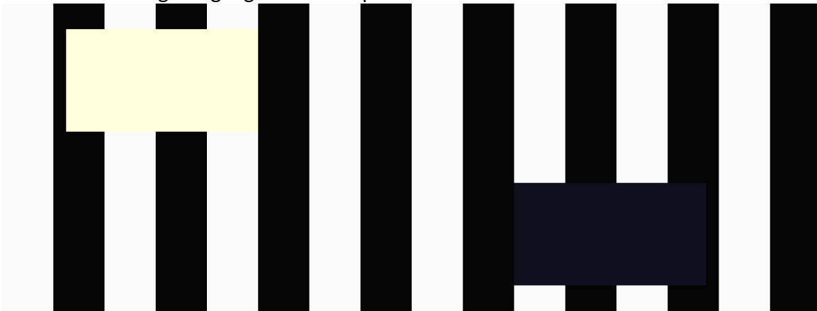
Sample Dynamic Range Stress frame: alternating bright/dark bars with extreme highlight and shadow regions.
